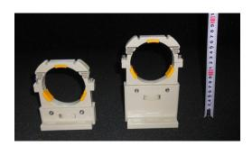
MMark & model : XGJ, The product is featured as easy operation and light weight. The elasticity of the product is capable to absorb the shaking caused by the transportation and protect the laser tube. The distance between the cross section center of laser tube in horizontal direction and the ground is about 80mm-90mm.
